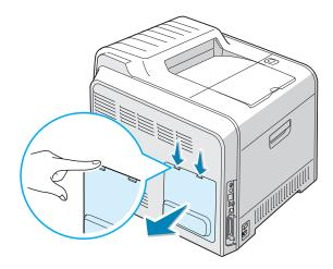
**3** Remove the two screws holding the metal plate in place, and then remove the metal cover, as shown below.
